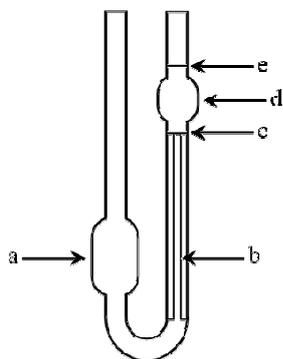
Fig. 1: A diagram of Ostwald viscosimeter. (a) lower bulb, (b) capillary bore, (c) lower mark, (d) upper bulb, (e) upper mark. (14).
