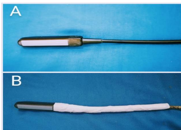
Figure 2: before and after applying the rubber tube to the probe.
