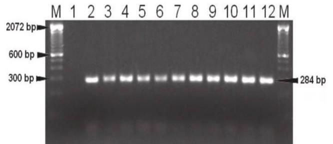
Figure 2: Gel electrophoresis for detection of *InvA* gene at 284 bp encoding *Salmonella Typhimurium* in artificially contaminated chicken meat. Image of PCR product running on 1.5 % of agarose gel for 90 minutes at 120V. M: DNA marker, Lane 1: Negative control, Lanes 2-12: Artificially positive samples.
